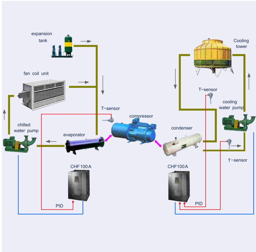
The difference of effluent temperature and backwater temperature of the water-cycling system in the central air-conditioning indicates the heat exchanger of the whole system needed. So, we can control the flow of water-cycling to control the heat exchange speed based on the difference, it is the first choice control mode for energy saving.
