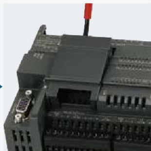
Remove the cover board with Screw driver
