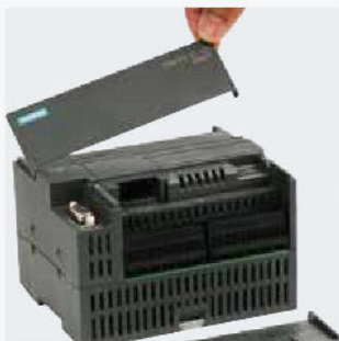
Remove the cover board of terminal
